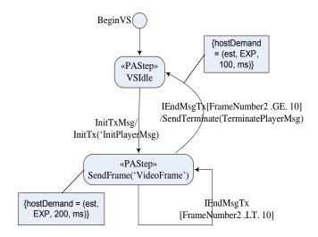
Figure 4. Video Server State Machine Diagram
