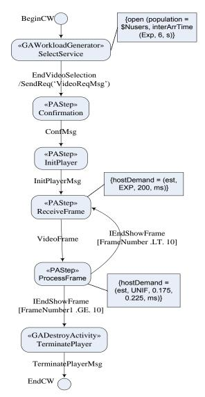
Figure 5. Client Workstation State Machine Diagram
