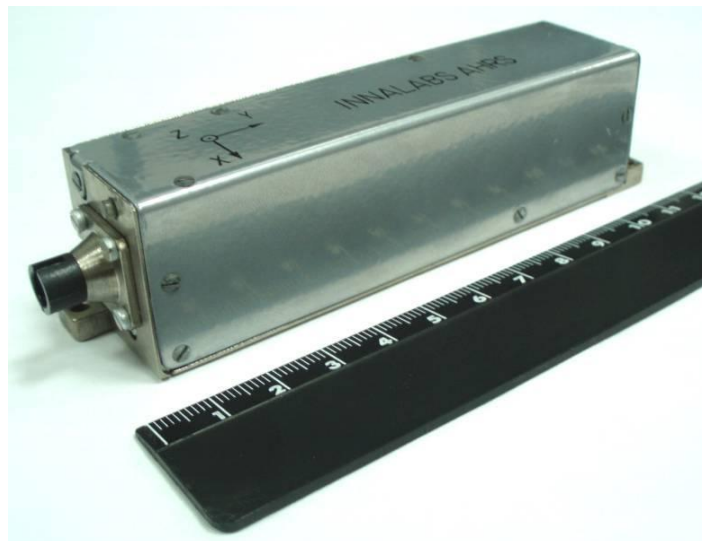
Figura 2.3 – Sensor AHRS da Innalabs (Innalabs, 2009).
