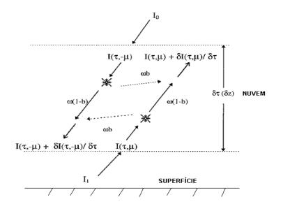
$$I(0,\mu) = \frac{I_1 + 2Ba^2\Omega(\mu) + I_0\Omega(\mu)(1-a^2)}{1+\Omega(\mu)(1+a^2)}$$
