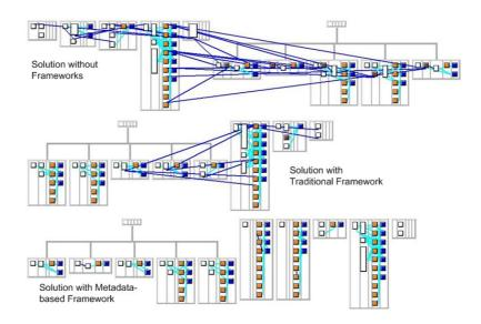
Fig. 2. Class Blueprint from the three implementations.
