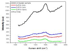
**Fig. 1.** Raman spectra for the untreated and treated carbon fiber samples.
