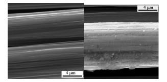
**Fig. 2.** SEM images of untreated (left) and N-PIII treated sample (right) for 10 minutes.
