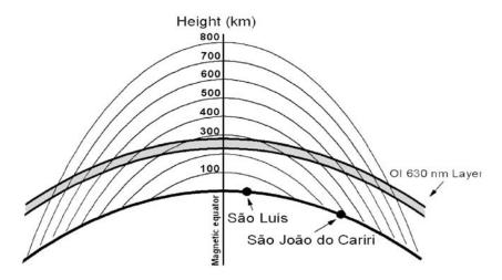
Figure 4. Geomagnetic field lines and Apex height over the geomagnetic equator. The shaded area indicates the OI 630.0 nm emission layer. Geomagnetic latitude of Cariri is around  $-11^{\circ}$ S.
