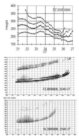
**Figure 3.** (top) Temporal variations of the true heights at the plasma frequencies, 10, 8, 5 and 1 MHz (from top to down), (middle) ionogram trace at 23:40 UT observed at Fortaleza, and (bottom) ionogram at São Luís at 23:40 UT on the night of September 30, 2005.
