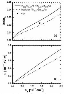
**FIGURE 2.** (a) The difference in occupation of the spinorbit split subbands in an InGaAs/InAlAs heterojunction (solid line) and insulator/InGaAs (dash line). (b) The  $\alpha$ parameter for both case. This is the paragraph spacing that occurs when you use the Enter key.
