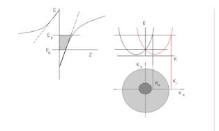
**FIGURE 1.** Scheme of the heterojunction and its constant electric field model, with the first subband occupied up to the Fermi energy; and, on the right, the scheme of the Rashba spin-orbit split, with the two Fermi wave vectors  $k_{\pm}$ .
