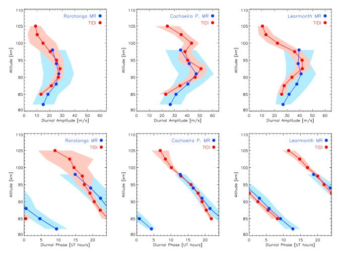
**Figure 2.** Height profiles (September–October 2005, first campaign) of the diurnal (top) amplitude and (bottom) phase (universal time of maximum) of the meridional wind for three stations and TIDI (60 day means) located at different longitudes near the 20°S latitude circle (see Figure 1 for the locations). Shading indicates standard deviation.
