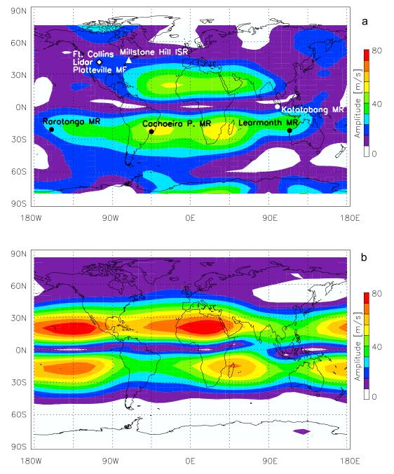
**Figure 1.** Latitude versus longitude cut of the net amplitude of the meridional wind (90 km, September 2005) of the diurnal tide reconstructed from the diurnal components diagnosed from (a) the TIDI observations and (b) the eCMAM. Results for the first campaign are shown.
